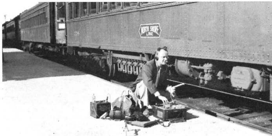
Recording compressor operation on North Shore car 724 at the Mundelein station. Note use of headphones.
